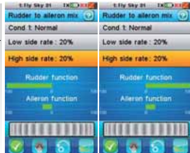
方向舵摇杆打到最左边 Rudder stick to the far left (Pic 21.8)
