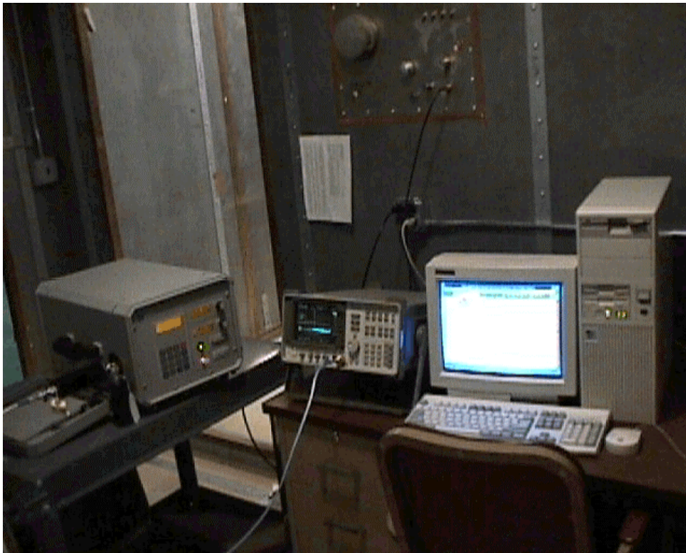
Photograph of Conducted Spurious Emissions and RF Power Output Test Configuration
