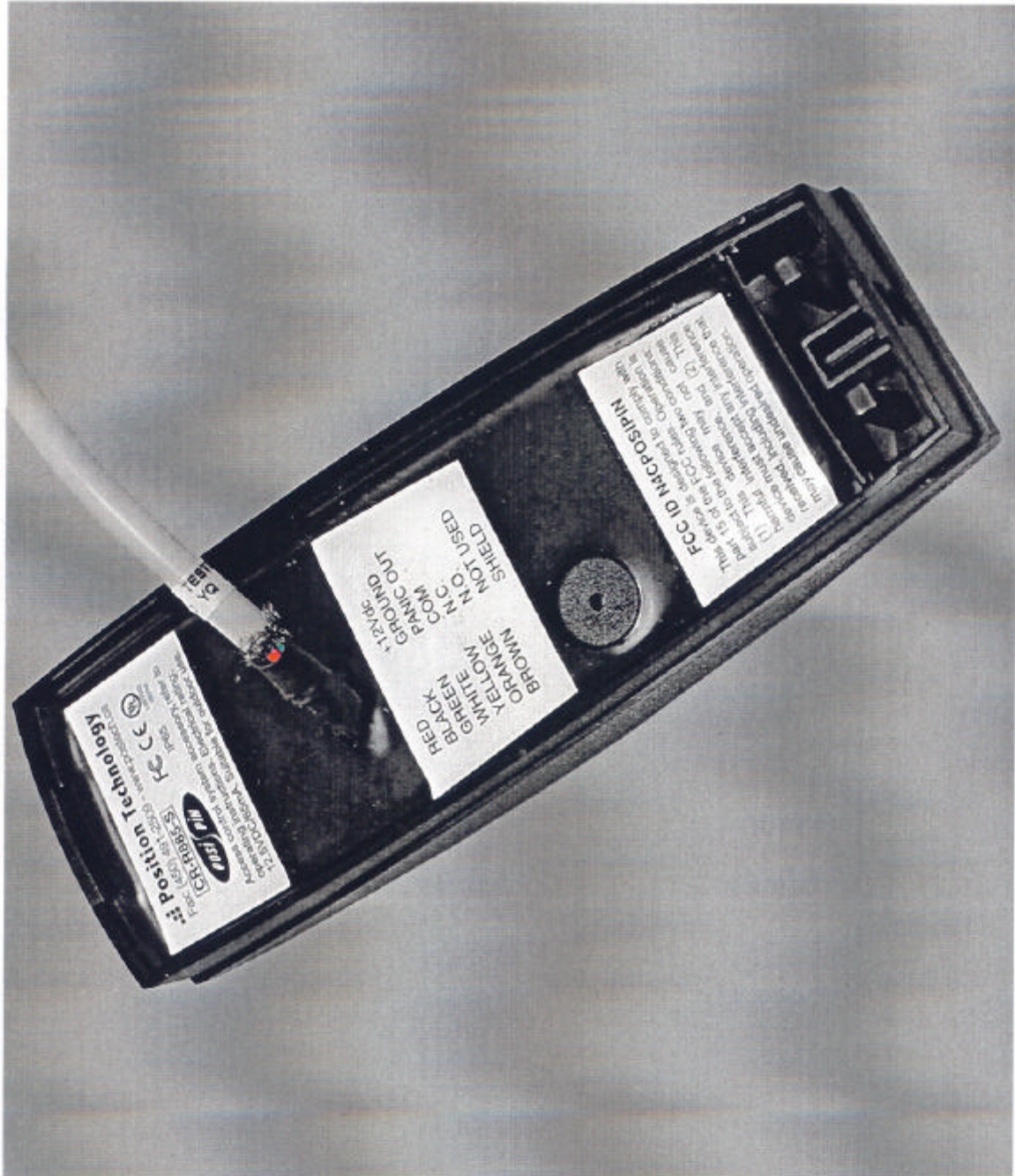
Rear external view with cover off (CR-R885S)
