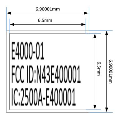
The inner frame is a label. The outer frame is an IC.
