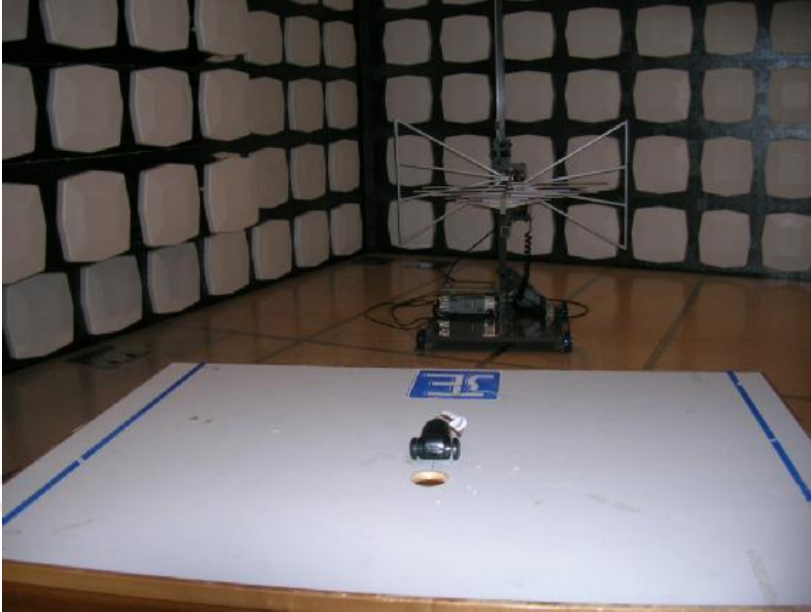
Measurement of Radiated Emission Test Set Up
