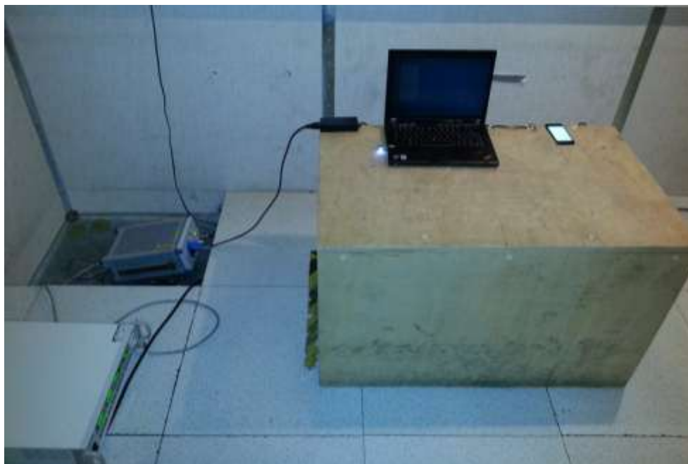
Test setup for power line conducted emissions
