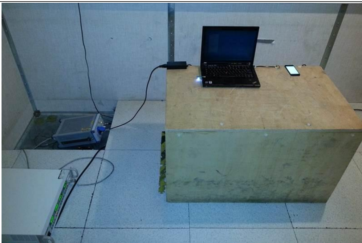
Photograph for AC Power Line Conducted Emissions (Global view)
