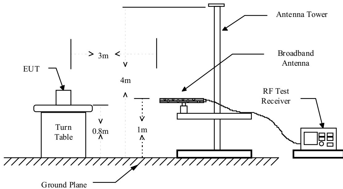
Radiated Emission's Frequency Above 1 GHz
