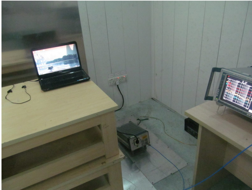
FCC RADIATED EMISSION TEST SETUP
