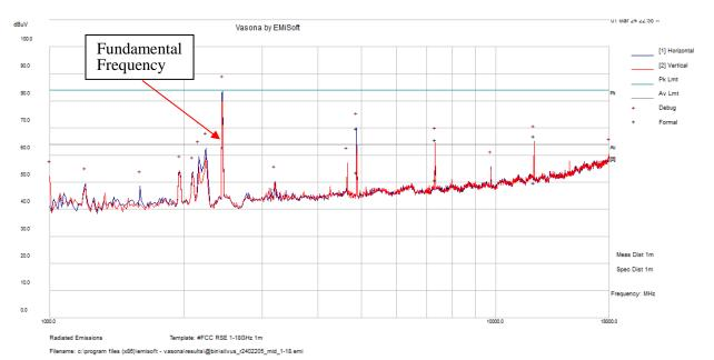
Antenna Turntable S.A. Correction Corrected Antenna **Frequency** Limit Margin Reading **Factor** Amplitude Height **Polarity Azimuth** Comment (MHz)  $(dB\mu V/m)$ (dB)(dBuV) (dB/m)  $(dB\mu V/m)$ (cm) (H/V) (degrees) 4878.8575 70.17 -0.34 69.83 140 Η 154 83.54 -13.71 Peak 53.98 -0.34 4878.8575 53.64 140 Η 154 63.54 -9.9 Average V 12198.193 60.63 6.46 67.09 191 103 83.54 -16.45 Peak 12198.193 43.32 6.46 49.78 191 V 103 63.54 -13.76 Average V 7318.875 63.06 2.61 65.67 110 168 83.54 -17.87 Peak
