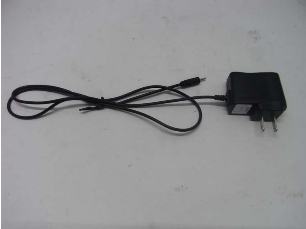
PHOTO OF POWER SUPPLY
