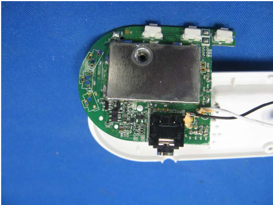
Parent Unit Main PCB comp side
