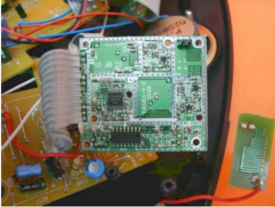
Base Oscillator PCB solder side
