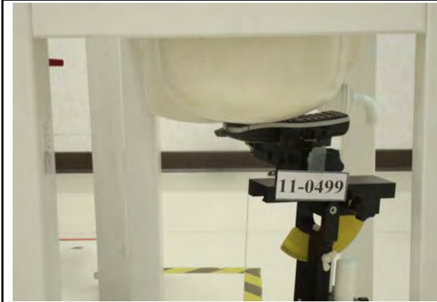
Figure 2. Right Head SAR Test Setup (Cheek)
