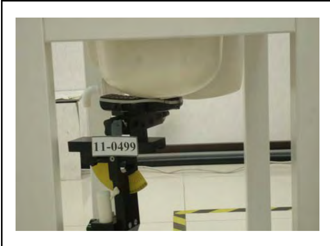
Figure 4. Left Head SAR Test Setup (Cheek)
