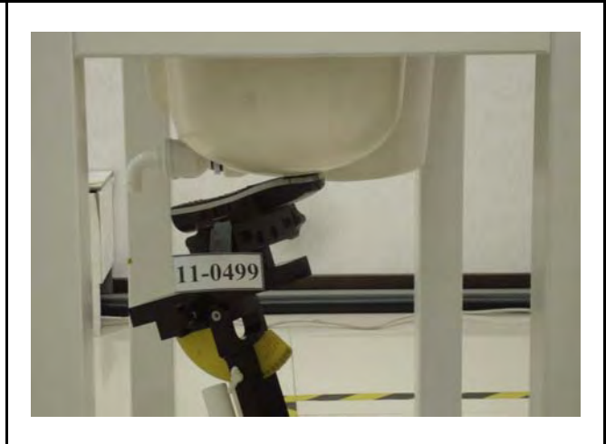
Figure 5. Left Head SAR Test Setup (Tilted)
