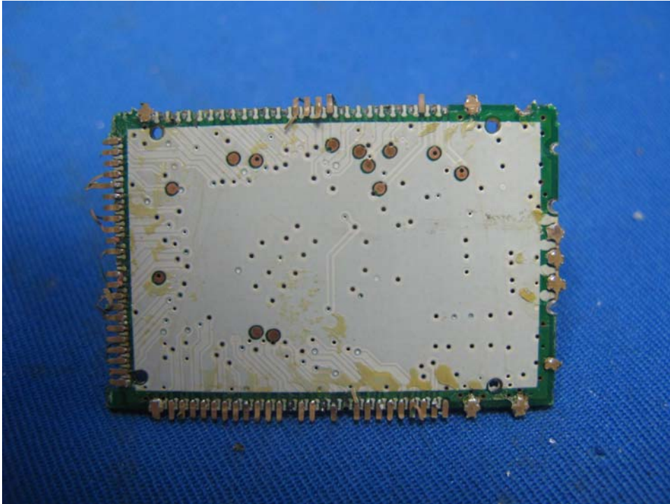
Base Unit DECT RF PCB solder side
