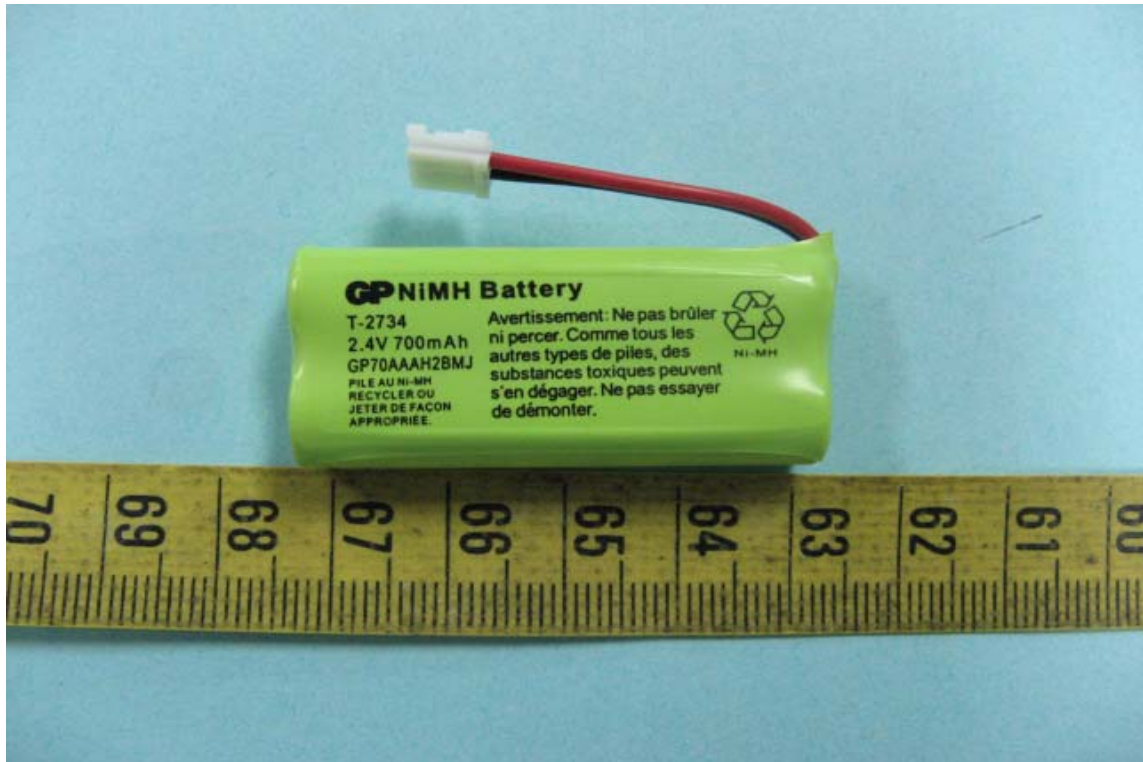
Front View of Battery
