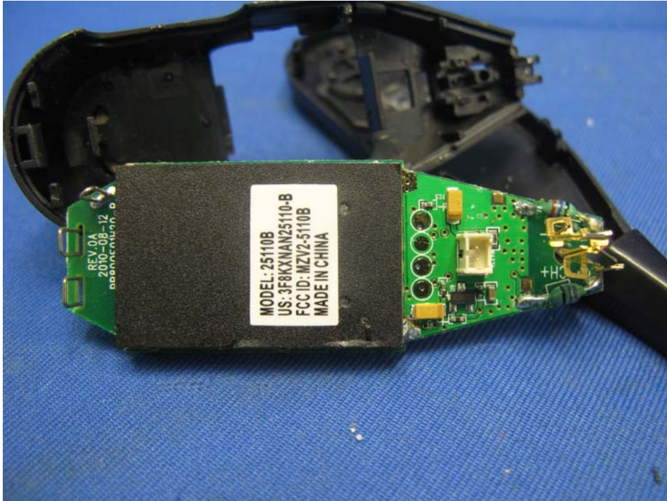
Headset Main PCB solder side
