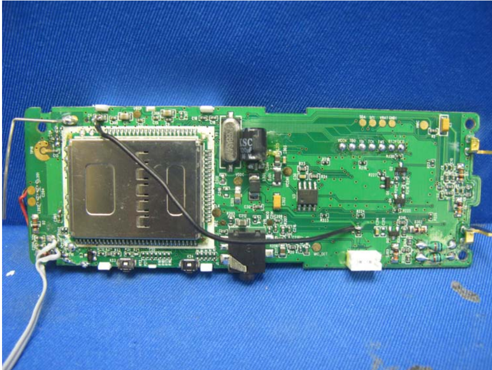
Handset Main PCB comp side (View 2)
