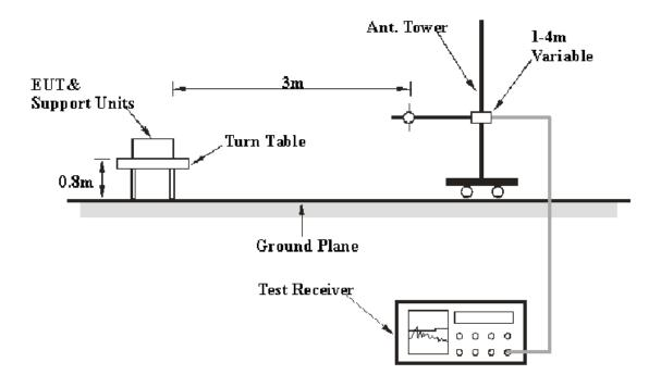
The deactivation test was performed in the 3 meters test site, using the setup accordance with the ANSI C63.4 - 2009. The specification used was the FCC 15.231(a) limits.
