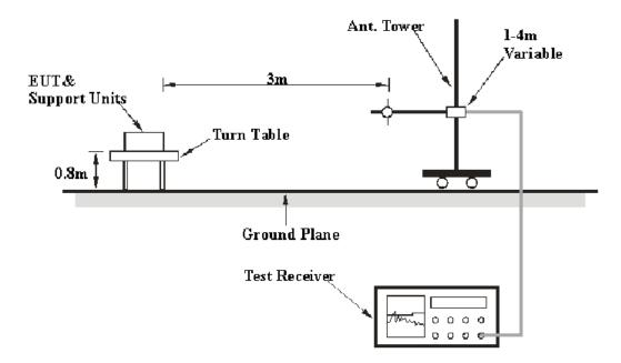
The radiated emission tests were performed in the 3 meters test site, using the setup accordance with the ANSI C63.4 - 2009. The specification used was the FCC 15 §15.209 and 15.231.
