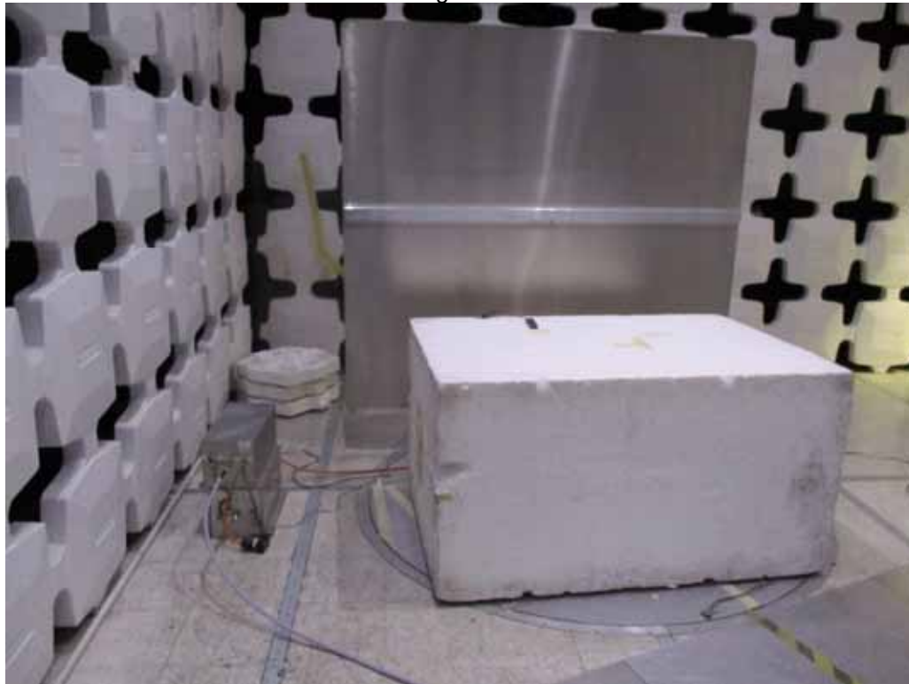
Test Setup for Conducted Emissions
