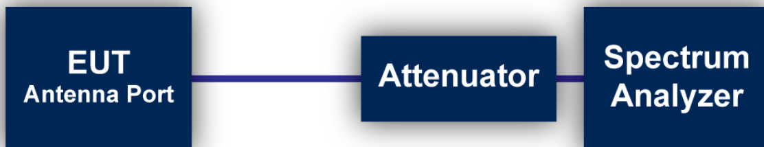
Figure 3: Direct Connection at the Antenna Port Test
