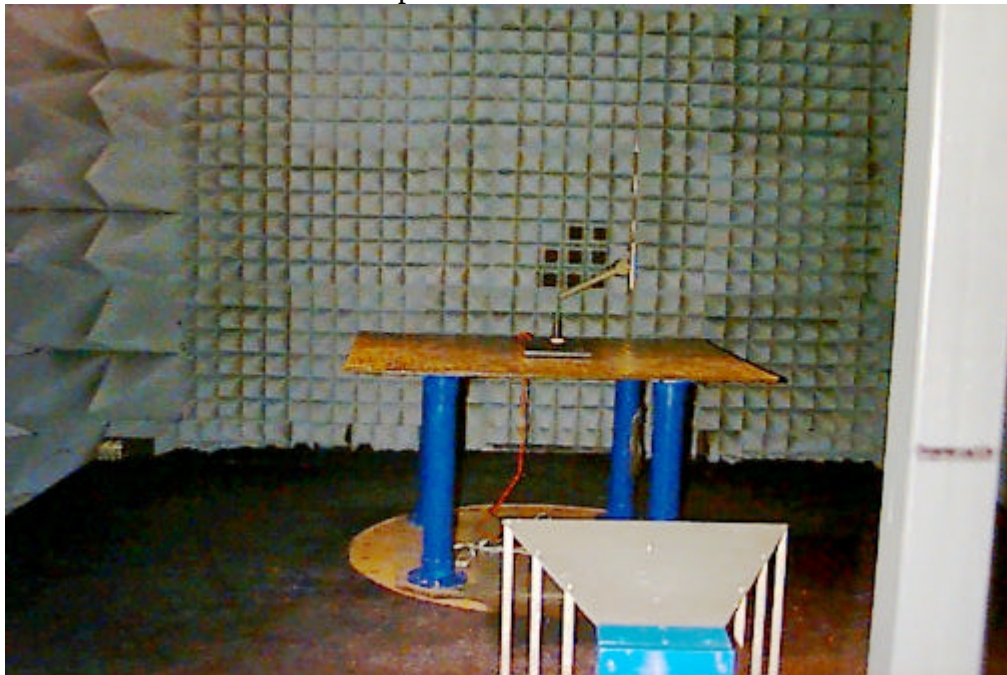
Dipole Antenna –Rear
