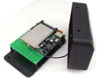
Connect the Pigtail Cable between the PC Card and the Amplifier/DC Injector input.
