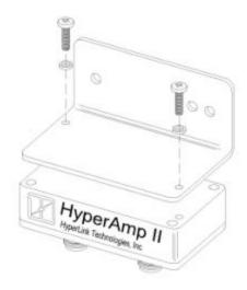
Install the right angle bracket as shown above using two (2) #10-24 screws and split lockwashers as shown. Note the orientation of the label relative to the 90 degree bend in the bracket. Proper positioning will ensure better visibility of the indicator LEDs when installed on the mast.
