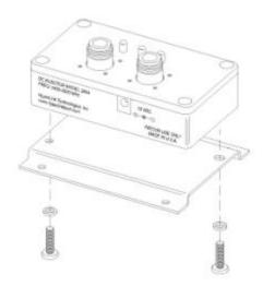
Install the bracket as shown above using two (2) #10-24 screws and split lockwashers as shown. For optimal lightning protection, it is recommended that one screw also be used for attachment of a suitable ground wire.
