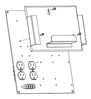
Attach the AC Power Cord to the Power Supply and clip the AP Power Supply into the base of the AP Mounting Bracket. Slide the AP module onto the mounting bracket. Make sure it is properly seated.
