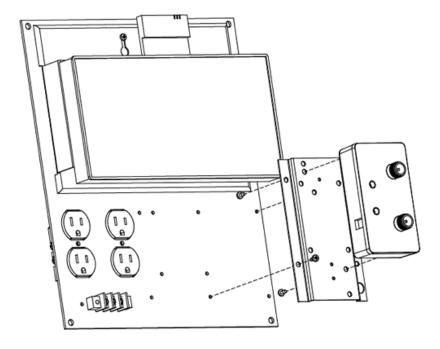
Connect the Pigtail Cable between the PC Card and the Amplifier input. Connect the amplifier output to the Filter/ Lightning Protector, as required (see Appendix A).
