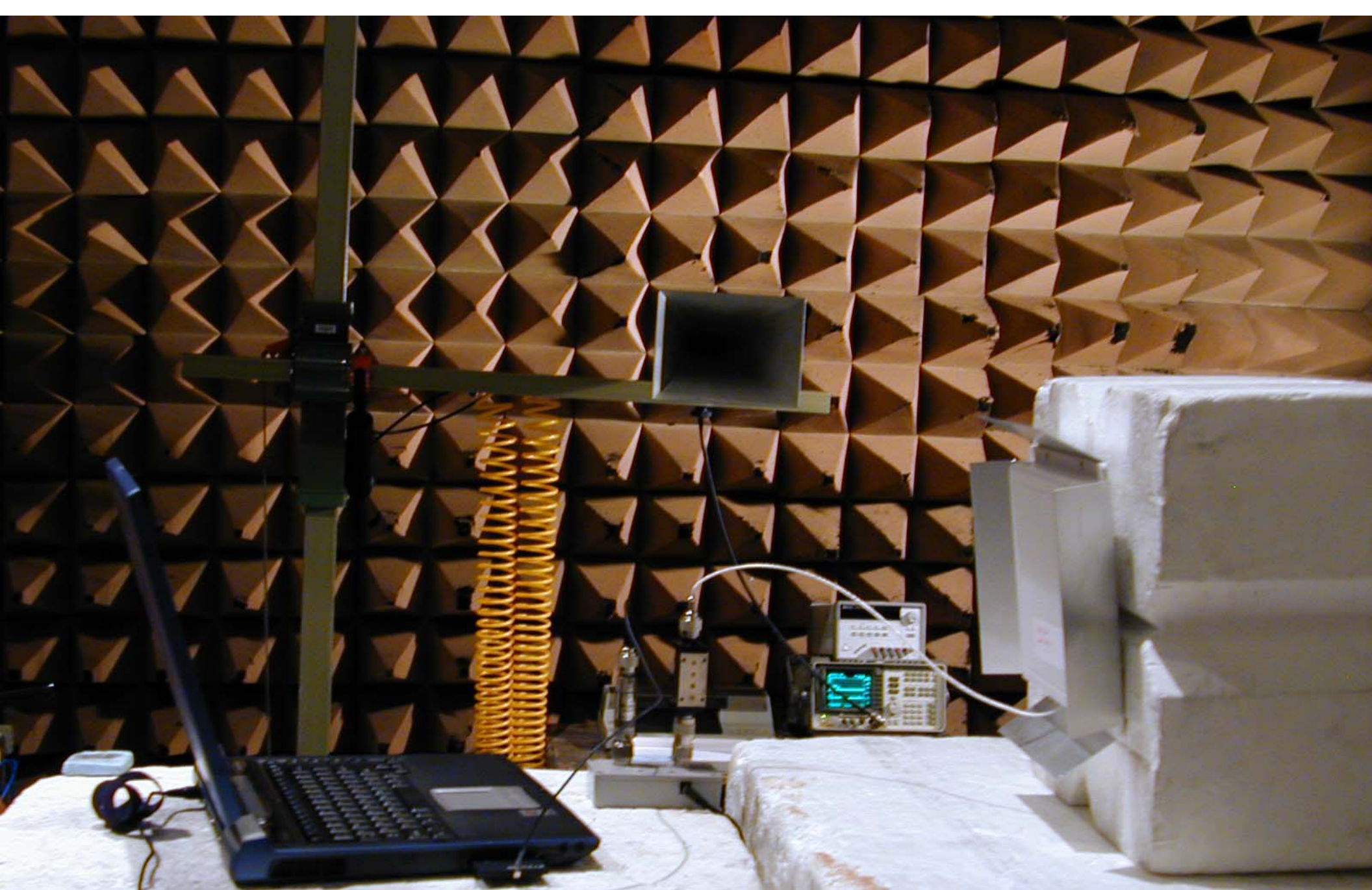
Radiated Emission Test Setup (HG2416P Antenna)
