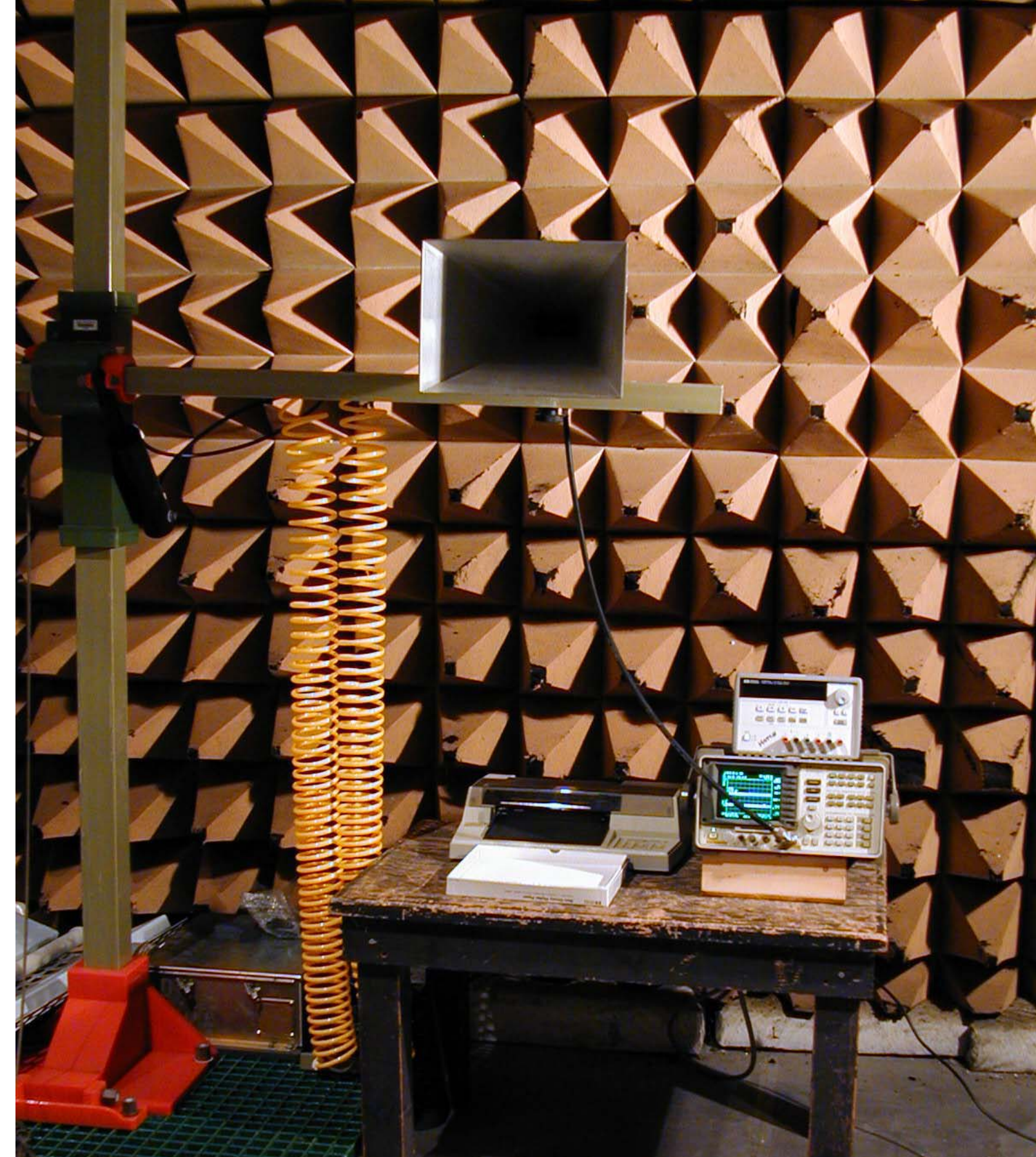
Radiated Emission Test Setup (Horn and SA)
