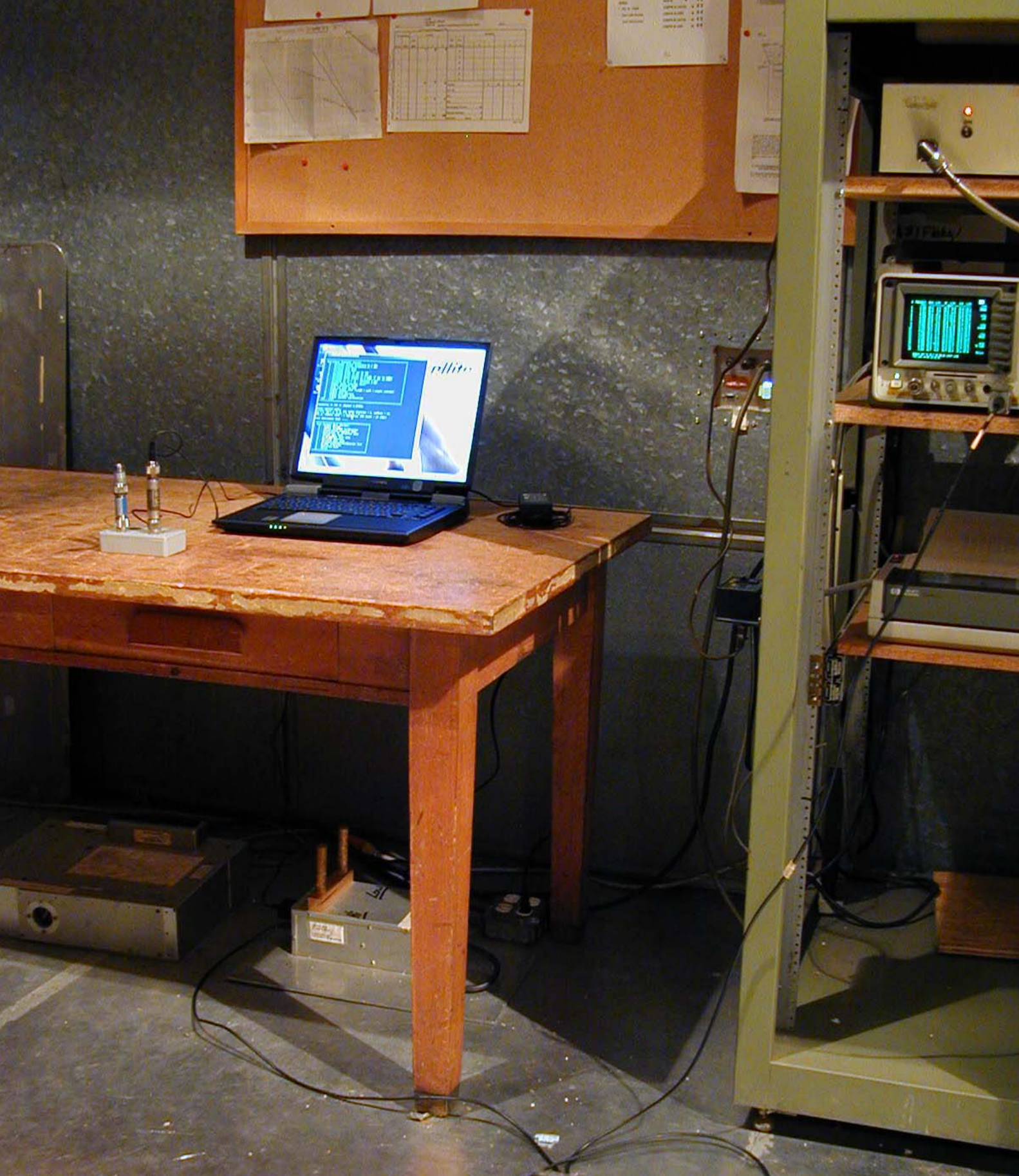
AC Line Conducted Emissions Test Setup
