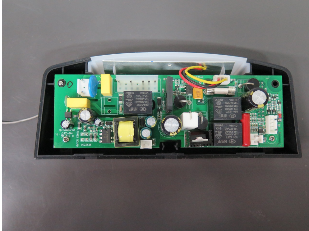
LQ-803 POWER BOARD
