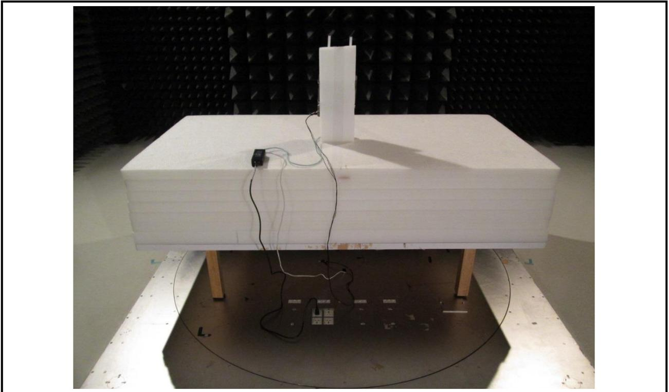
**Radiated Emission Above 1GHz Test**
