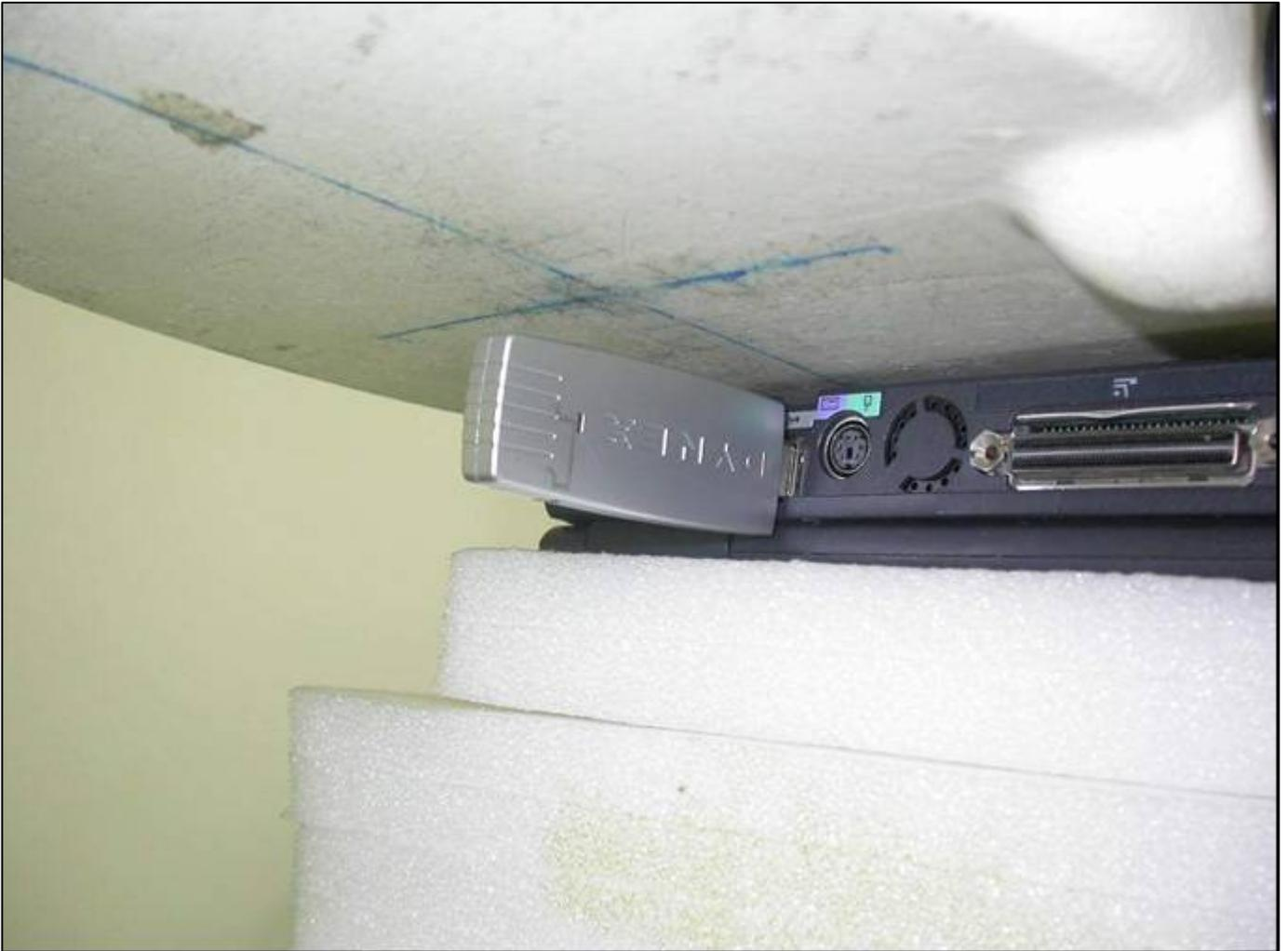
**The edge of the EUT to the flat phantom distance 7 mm**
