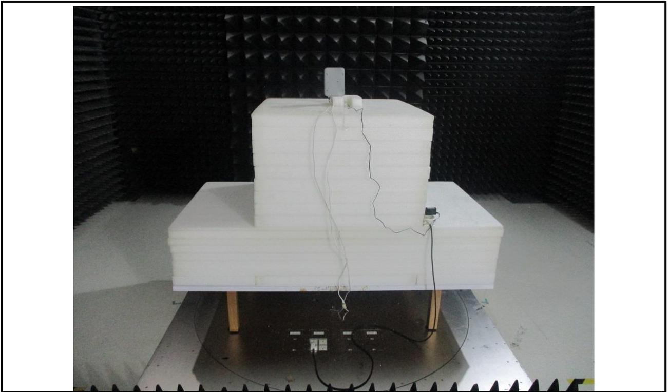
**Radiated Emission Above 1GHz Test**
