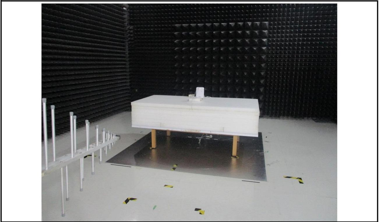
**Radiated Emission Above 1GHz Test**
