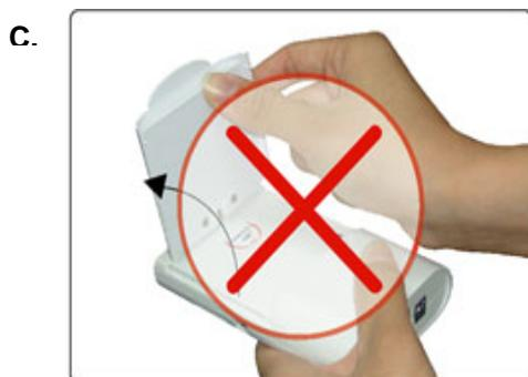
The antenna housing can rotate up to 135 degrees clockwise/counter-clockwise (See pictures D-G). It will be locked /lodged in every increment of 45 degrees in position.
