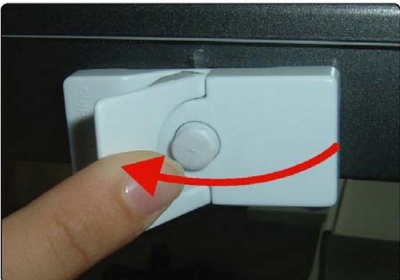
3. To Grasp and lift the salient part of the suction cap to allow ventilated. So, USD can be easily torn off. (See pictures D&E )
