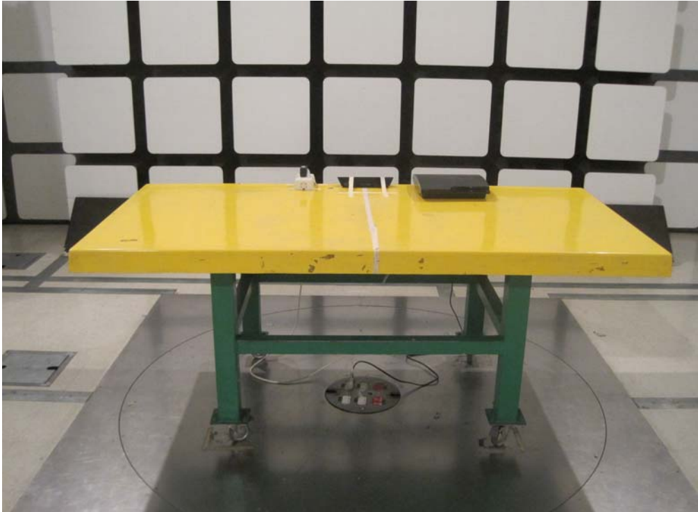
Radiated Emissions from 30 MHz to 1GHz
