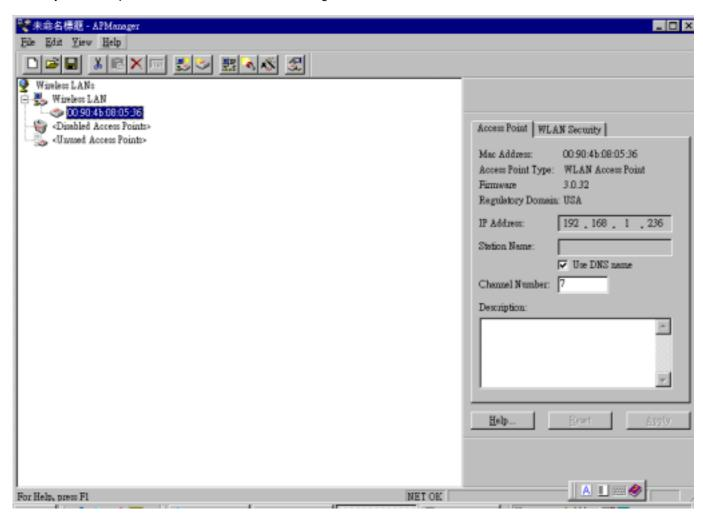
The tree structure on the left of the window shows a list of WLANs (Wireless LANs) and the Access Points that are part of each WLAN. The sample image above shows a single Access Point with hardware address 00:90:4b:08:05:36 that is assigned to the WLAN named "Wireless LAN". The icons indicate the status of the WLANs and their associated Access Points.
