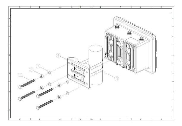
The IOT Macro Gateway can also be mounted on a wall. It comes with mount kit as shown here:
