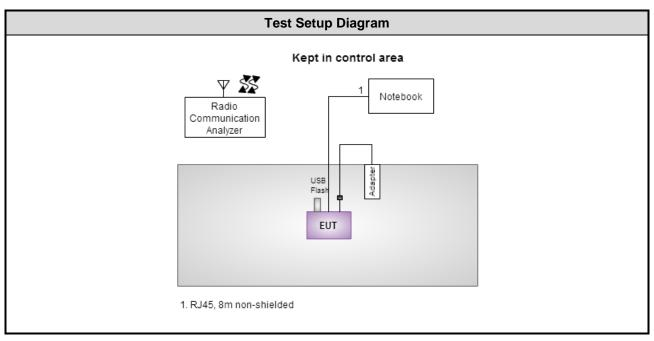
Note: The module is certified as limited module that is limited to specific host (refer to section 1.1.2). Thus, test configuration is combined with host not stand-alone
