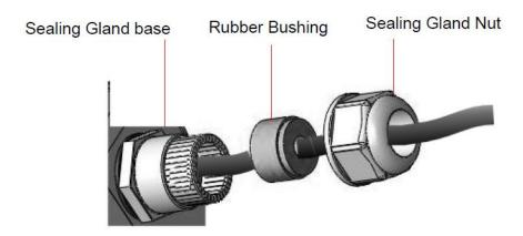
Tighten the gland nut. Use the dedicated tool for fastening the sealing glands.
