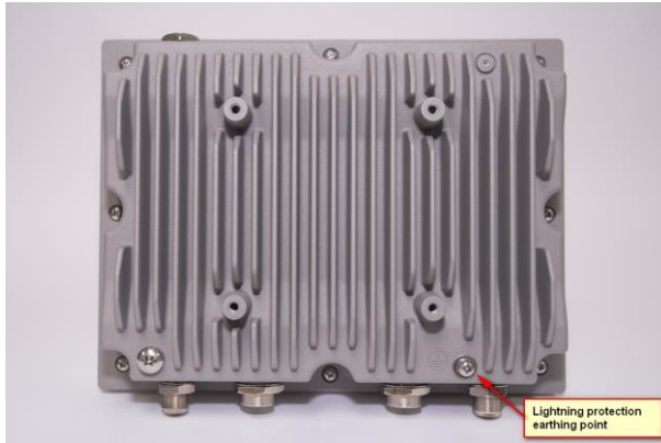
Figure 6 - Lightning protection earthing point
