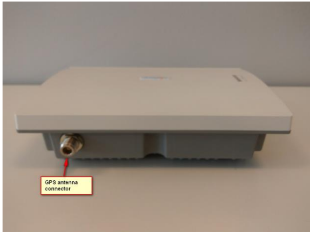
Figure 4: GNSS antenna port
