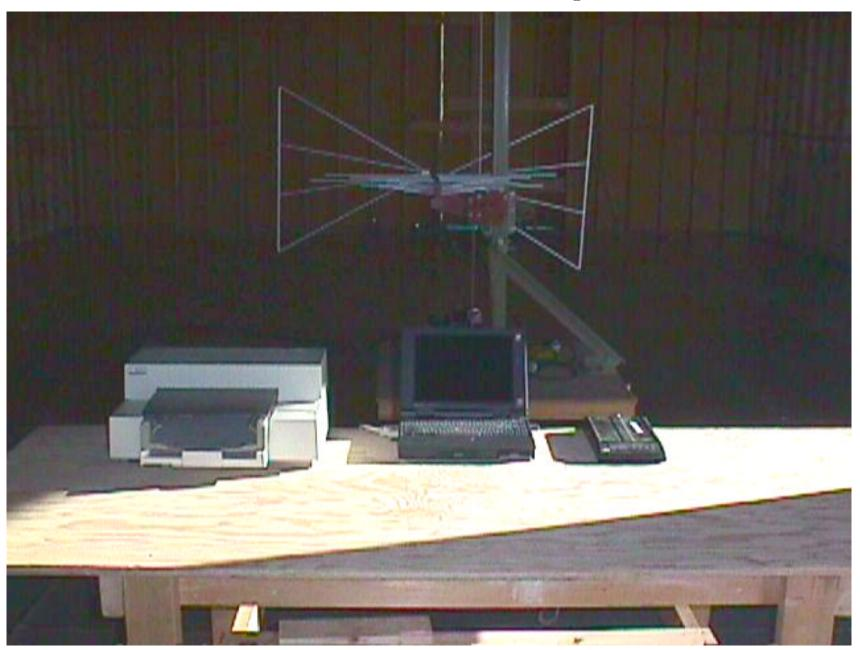
**Transmitter Radiated Emissions Test Setup (Front View)**
