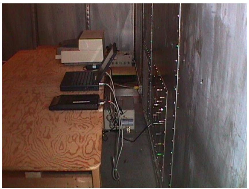
AC Powerline Conducted Emissions Test Setup (Side View)
