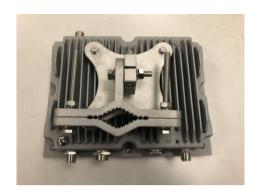
Step 5.Install the device on a pole.
