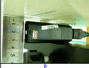
The left edge of the EUT faces to the phantom with 5mm-separation distance.
