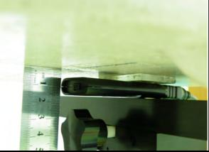
The front of the EUT faces to the phantom with 5mm-separation distance.
