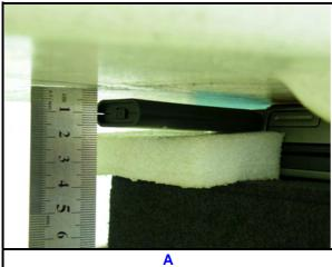
The bottom of the EUT faces to the phantom with 5mm-separation distance.
