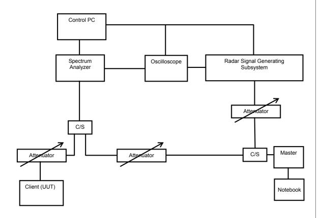
The UUT is a U-NII Device operating in Client mode without Radar Detection function. The radar test signals are injected into the Master Device.
