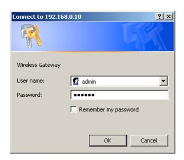
In order to configure the Wireless SOHO AP Router, you must input the username into the **User Name** box. Enter the password into the **Password** box and press the **OK** button. The default User Name is "admin". There is no default password, leave the Password field blank.
