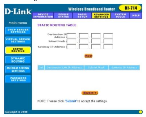
In Static Routing, the user has the ability to add a static route to the routing table by simple entering the destination IP, subnet mask, and gateway. Clicking on "Add" and then "Submit" which requires a restart for the IP address to be incorporated into the routing table.
