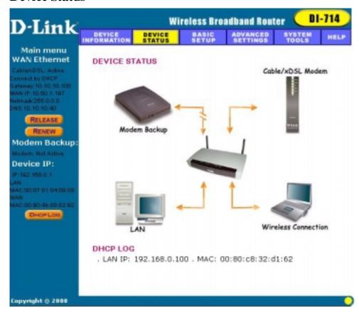
The Device Status screen displays a graphical representation of your current configuration. The left side of the screen shows your connection information in regards to WAN and LAN IP Address information. The right side displays the connection status of each device.
