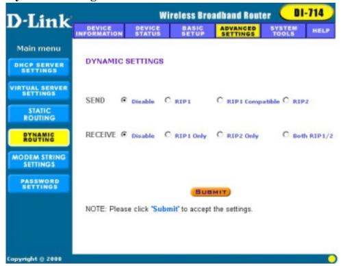
By default, the Broadband Router will not send or receive any routing Internet protocols (RIP) to update the routing table. However, the user can enable the Broadband Router to automatically send and receive RIP packets to establish routes for commonly used paths.
