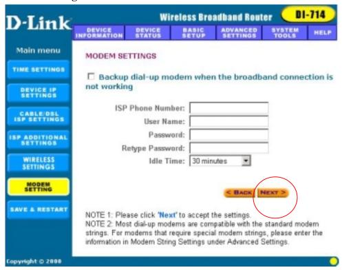
An analog external modem can be used as a dialup backup to the DSL/Cable connection. If you would like to use a modem backup, you need to enable the modem settings function. Click on "Modem Settings" on the left hand side and input the ISP account settings.
