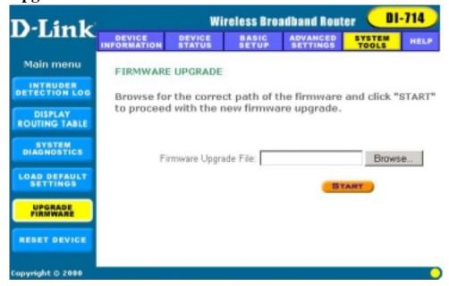
The Upgrade Firmware screen enables you to update the firmware used in the DI-714. Visit D-Link's product support site (www.dlink.com) to download an updated firmware. Firmware updates usually fix problems encountered by users, and may incorporate new features.
