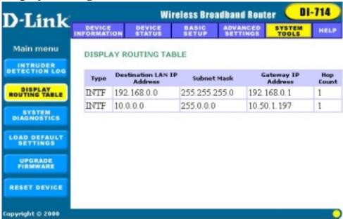
The Display Routing Table screen displays the routing table that the DI-714 is using. A router uses a routing table to keep track of what IP addresses there are and where the router should forward packets when it receives them.
