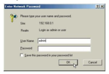
In order to configure the DI-714 you must input the user-name into the **User Name** box. Enter the password into the **Password** box and press the **OK** button. The default User Name is "admin." There is no default password, leave the Password field blank.
