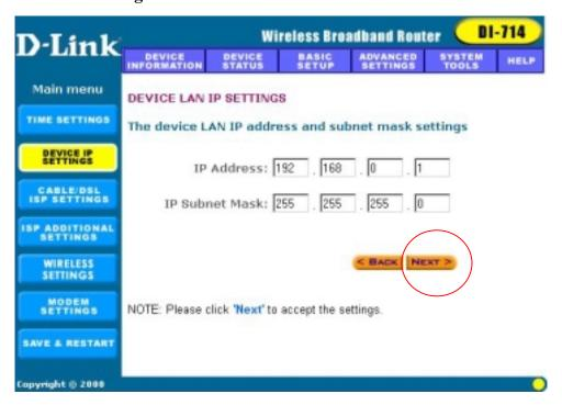
You have to give your Internet gateway an IP address on your "private" network. This is not the "public" IP address from your ISP but the local internal LAN IP address. The IP address of "192.168.0.1" is the default IP address of the LAN port in the broadband router.
