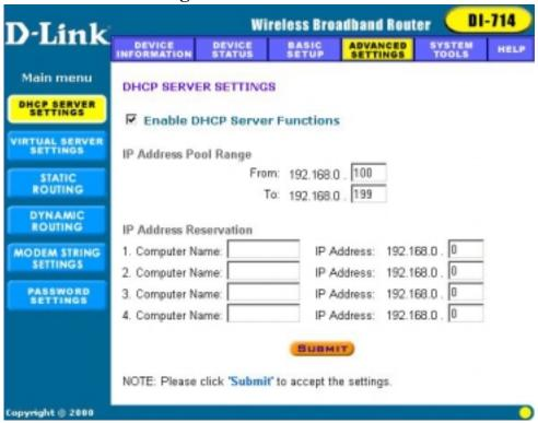
By default, the Broadband Router has DHCP server enabled to assign an IP address ranging from 192.168.0.100 to 192.168.0.199. In addition, the router is capable of reserving up to four IP addresses within the local network for mail, web, or ftp server.
