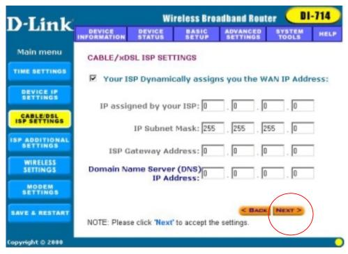
The DSL/Cable ISP settings have a default to obtain dynamically the IP address for the WAN port of the broadband router. Some ISPs may give you Static IP settings. If this is the case for your ISP then you need to:
