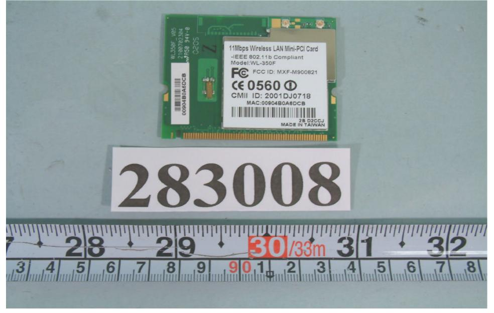
Wireless LAN Mini-PCI Card With The Shield Removed
