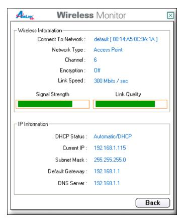
If you do not have adequate Signal Strength, try re-orienting the Access Point and/or the antennas of PCI Adapter to get a better reception.
