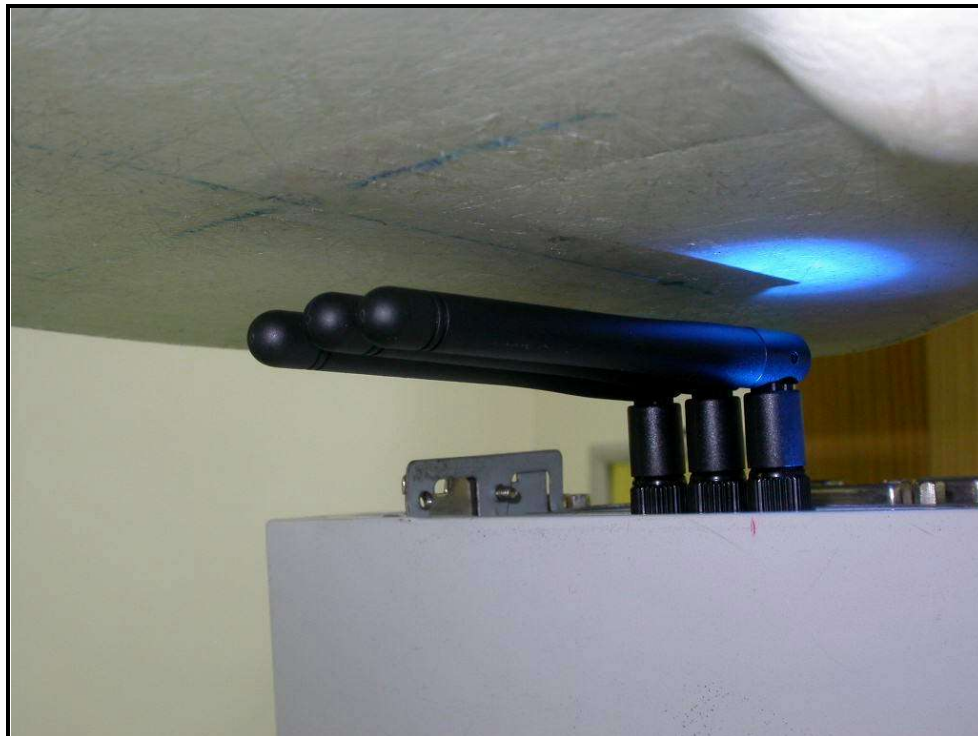
The bottom of the EUT face to the phantom with 5 mm-separation distance.
