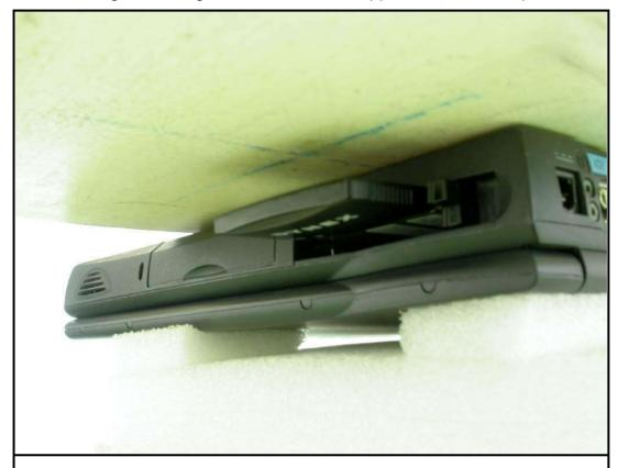
The bottom of the EUT face to the phantom with 12mm-separation distance.
