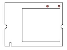
Your computer comes with a unique Mini PCI Card socket, which allows the computer to add wireless LAN (IEEE802.11g).
