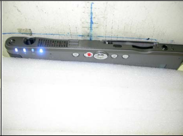
B: The bottom of the EUT (side of antenna 2) face to the phantom with 0mm-separation distance.
